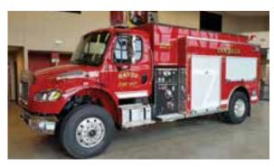
Freightliner M2 106 chassis, 350HP Cummins ISL diesel engine, Allison 3000EVS transmission, NFPA Enhanced Stability Control, On-Spot chains, Darley 500gpm pump with pump and roll capability, NFPA 2430gal T Style poly tank, 10" Newton rear dump chute, Hanney compartment mounted 150' electric hose reel, Whelen lighting/siren/air horn systems.
